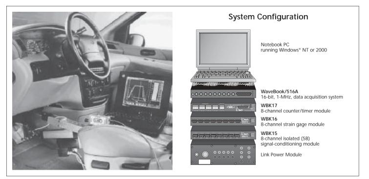
Link has integrated IOtech data acquisition components into its vehicle component test machines and vehicle test systems because of its modularity, flexibility, and high reliability. Mobile systems are used in vehicles for investigating noise, vibration, and harshness (NVH); correlating brake noise to other parameters; analyzing data; and general troubleshooting.
